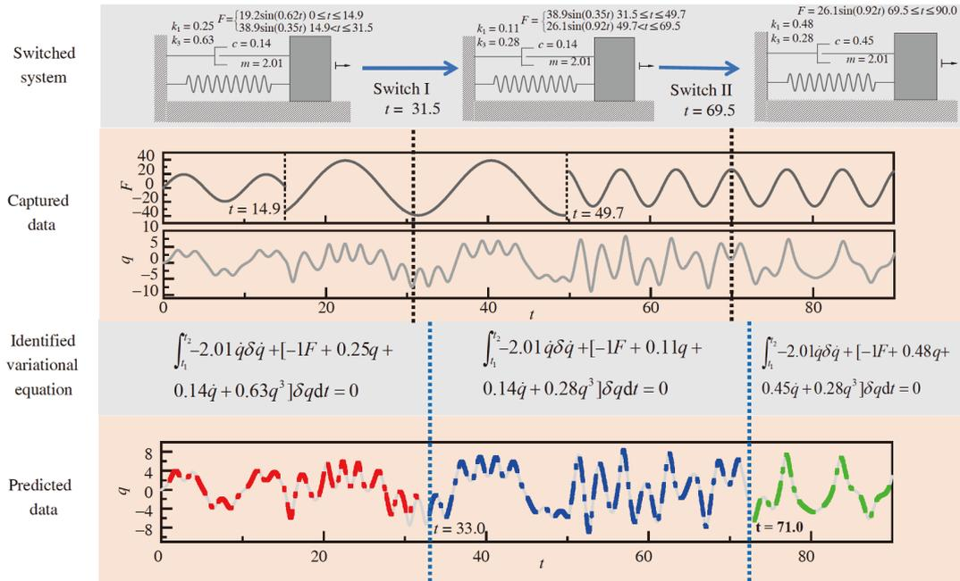
**Figure 2** (Color online) Demonstration of the switched Duffing oscillator with sinusoidal excitation. First row: physical model of Duffing oscillator with preset values of system parameters and moments of switches; second row: captured data of sinusoidal excitation and state variables with sampling frequency 0.001 s; third row: identified variational equation for each stage; fourth row: comparison of predicted trajectory and captured data.
