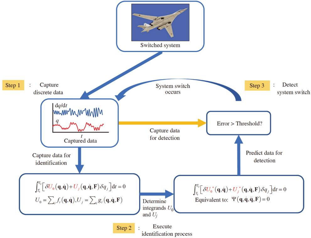
**Figure 1** (Color online) Flow chart of the proposed methodology. The whole process consists of three successive steps: step 1, capture the discrete data in real time; step 2, identify the variational equation governing the dynamic behaviors of the switched system; step 3, detect the occurrence of switches ceaselessly, and reidentify the renewed variational equation once a switch occurs.
