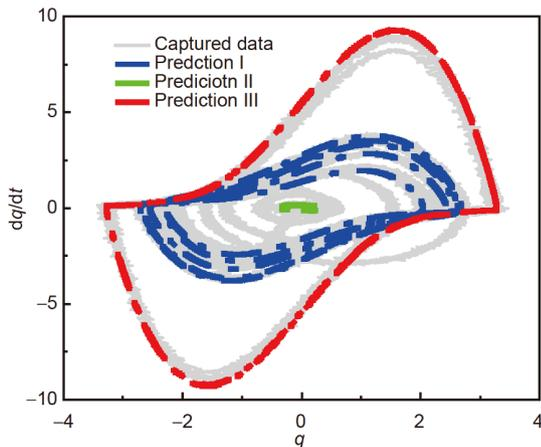
**Figure 9** (Color online) Comparison of predicted phase diagram to captured phase diagram for switched van der Pol system with sinusoidal excitation (noise intensity 0.05, and integral interval 24 s).
