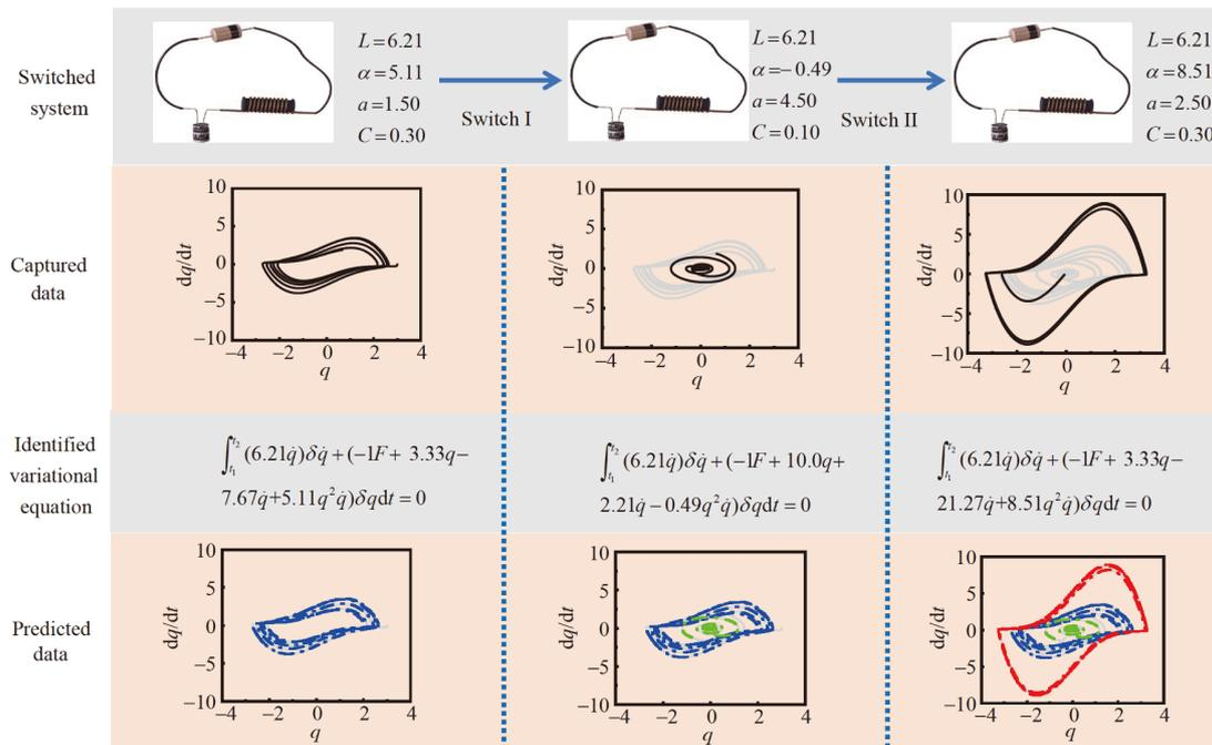
**Figure 6** (Color online) Demonstration of the switched van der Pol system with sinusoidal excitation. First row: physical model of van der Pol system with preset values of system parameters and moments of switches; second row: captured phase diagram with sampling frequency 0.001 s; third row: identified variational equation for each stage; fourth row: comparison of predicted phase diagram and captured phase diagram.
