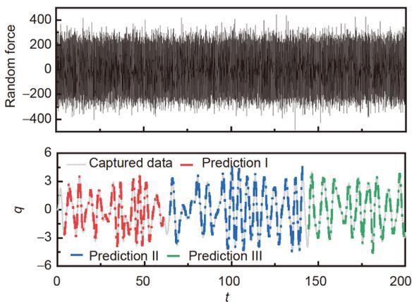
**Figure 3** (Color online) Demonstration of the switched Duffing oscillator with random excitation. Top row: captured discrete data of random excitation; bottom row: comparison of predicted trajectory and captured data.
