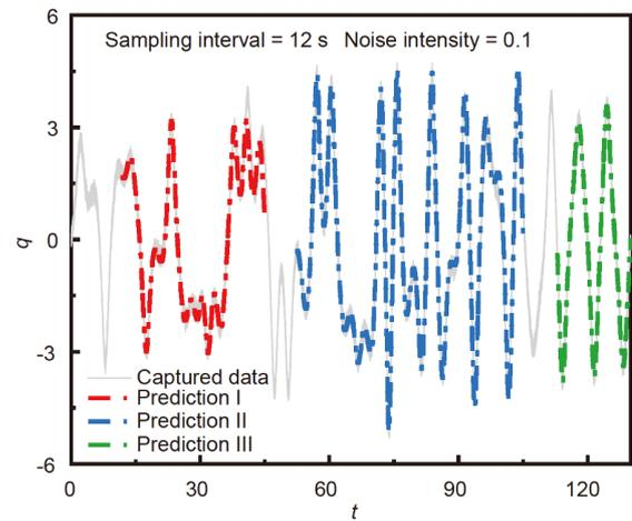
**Figure 5** (Color online) Comparison of predicted trajectory to captured data for switched Duffing oscillator with sinusoidal excitation (noise intensity 0.1, and integral interval 12 s).
