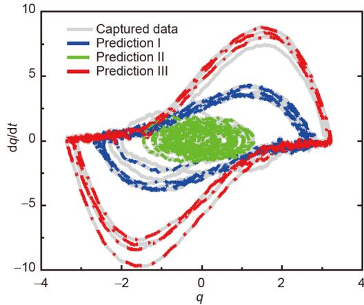
**Figure 7** (Color online) Comparison of predicted phase diagram with captured phase diagram for switched van der Pol system with random excitation.
