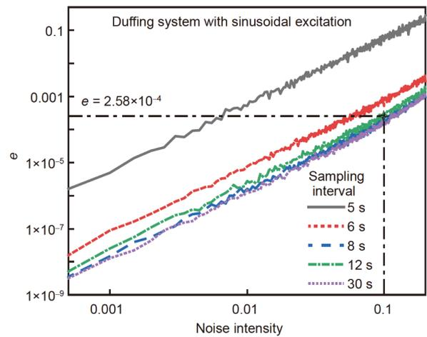
**Figure 4** (Color online) The relation of the relative error of Duffing oscillator with sinusoidal excitation to the noise intensity for five different integral intervals.
