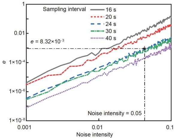
**Figure 8** The relation of the relative error of van der Pol system with sinusoidal excitation to noise intensity for five different integral intervals.
